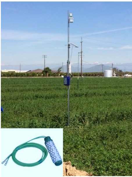
Fig 6. Wireless soil moisture monitoring network
