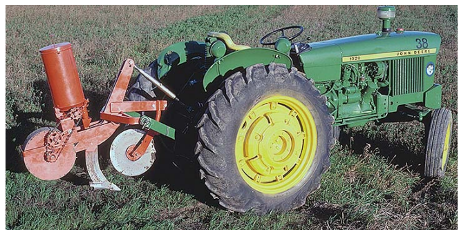
A 10.2. (A) A tractor-drawn mechanical bait applicator is useful for large areas. (B) It constructs an artificial burrow and deposits poison grain at preset intervals.
