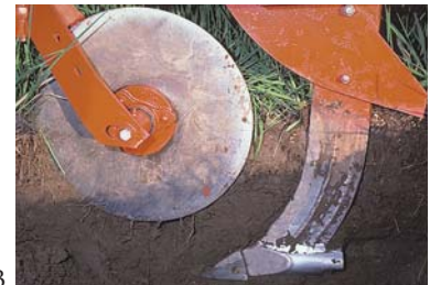
A 10.2. (A) A tractor-drawn mechanical bait applicator is useful for large areas. (B) It constructs an artificial burrow and deposits poison grain at preset intervals.
