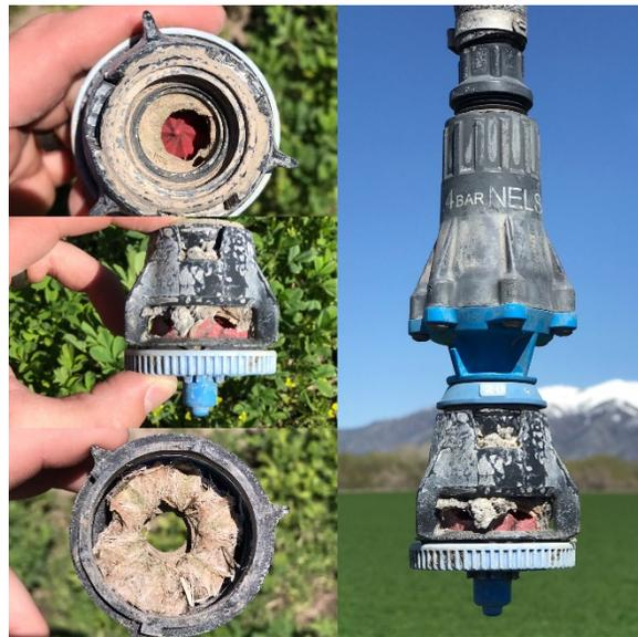
Figure 1. Moss debris clogging pivot sprinkler.
