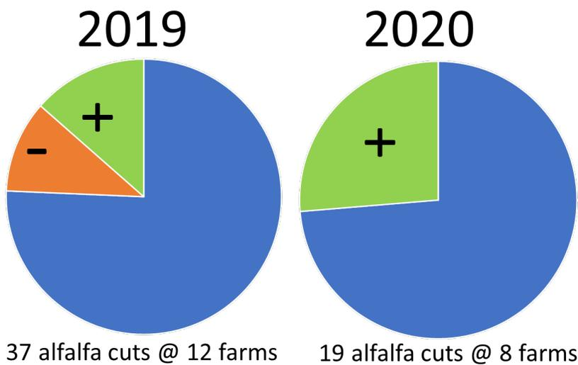
**Figure 6.** Summary of the impact of new sprinklers on alfalfa yield at test fields in 2019 and 2020. Green (+) indicates that yield was improved, orange (-) indicates a reduction in yield, and blue was no impact on yield.
