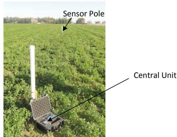
**Fig. 1. The water arrival sensing and communication system**
