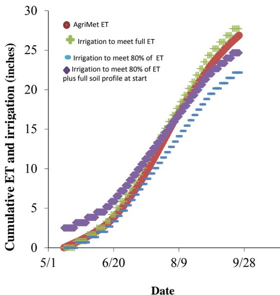
**Figure 4.** Irrigation system performance relative to AgriMet-estimated, 30-year average corn ET, Kimberly, ID. Assumed center pivot capacity is 0.28 inch/day with net irrigation of 6.5 gpm/acre at 80% application efficiency.
