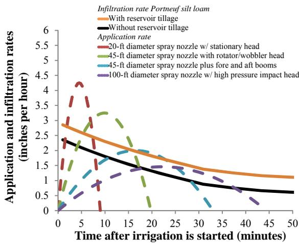
**Figure 15.** Estimated water application rates from three sprinkler devices under the last (outer) pivot span and from the 45-foot-wetted-diameter device with alternate fore-aft booms as compared with the infiltration rates with and without reservoir tillage for a Portneuf silt loam soil.
