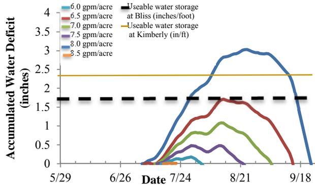
**Figure 9.** Accumulated water deficit (AgriMet ET - water applied) with center pivot capacities of 6–8.5 gpm/acre, Kimberly, ID, 2006.
