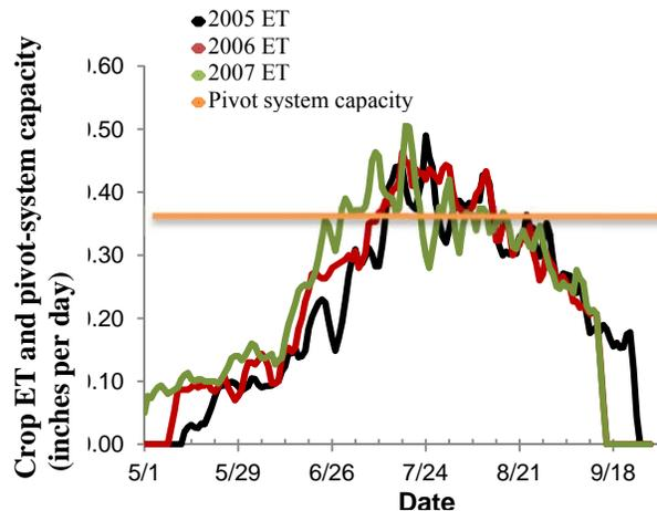
**Figure 7.** AgriMet-estimated crop water use and pivot system capacity for corn at Bliss, ID. ET data are plotted as a 3-day moving average to smooth daily fluctuations.
