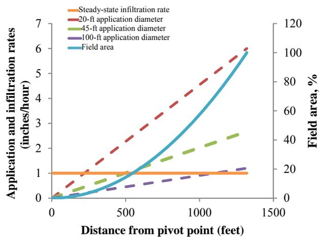
**Figure 16.** Steady-state infiltration rate on a sandy loam soil, sprinkler application rate, and percentage of field area with distance from pivot point.
