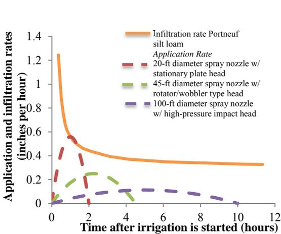
**Figure 11.** Estimated water application rates from three sprinkler devices under the first pivot span as compared with the infiltration rate for a Portneuf silt loam soil, Kimberly, ID.
