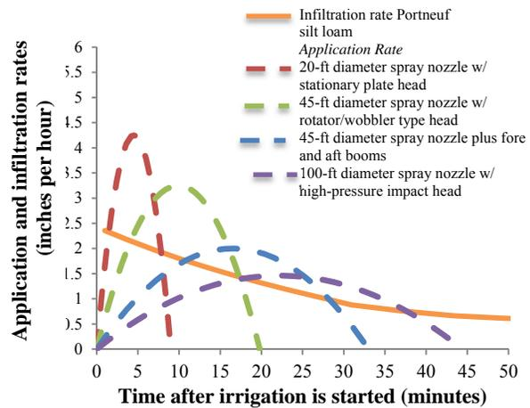
**Figure 12.** Estimated water application rates from three sprinkler devices under the last (outer) pivot span and from the 45-foot-wetted-diameter device with alternate fore-aft booms as compared with the infiltration rate for a Portneuf silt loam soil, Kimberly, ID.
