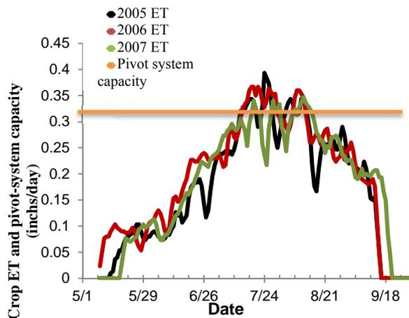
**Figure 6.** AgriMet-estimated crop water use and pivot system capacity for corn at Kimberly, ID. ET data are plotted as a 3-day moving average to smooth daily fluctuations.
