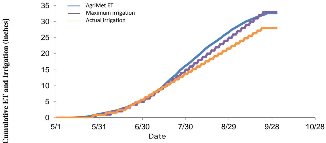
**Figure 3.** AgriMet-estimated cumulative corn ET, Bliss, ID 2005, and the actual cumulative irrigation applied. The maximum irrigation curve represents net center pivot irrigation system capacity at 7 gpm/acre and 85% application efficiency.
