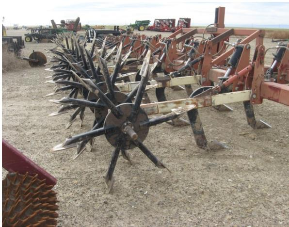
**Figure 13.** Dammer Diker equipment for row crops.
