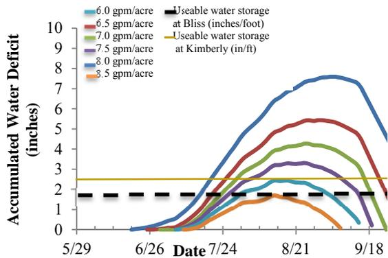
**Figure 8.** Accumulated water deficit (AgriMet ET - water applied) with center pivot capacities of 6–8.5 gpm/acre, Bliss, ID, 2006.
