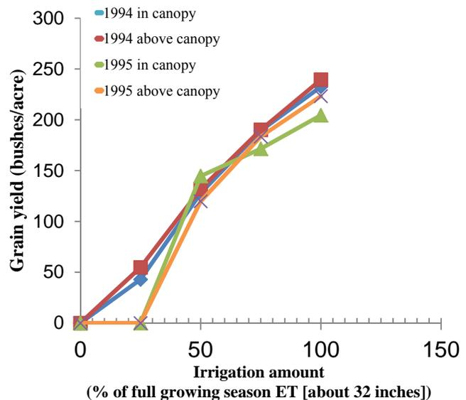
**Figure 5.** Grain yield response to irrigation treatment, Bushland, TX, 1994 and 1995. (Source: Schneider, A. D., and T. A. Howell. 1998. LEPA and spray irrigation of corn—Southern High Plains. *Trans. ASAE* 41(5):1391–1396.)
