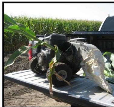
**Step 2.** Hand feed the plant to a **chopper** (you can use a chipper shredder).
