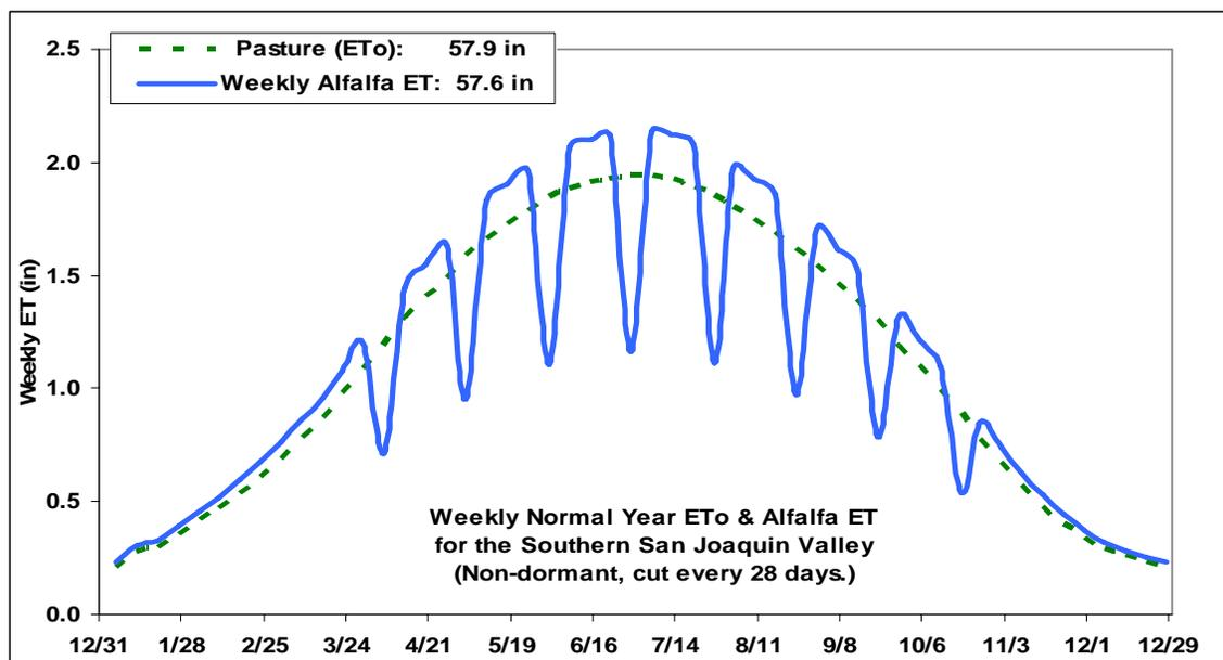
Fig. 2. Weekly ET for an established stand of non-dormant alfalfa in the SJV with 8 cuttings. Crop ET is calculated using peak crop coefficient (Kc) values of 1.1 immediately upon irrigating after bale pickup and a low of 0.6 for one week immediately after cutting as the hay cures prior to baling.
