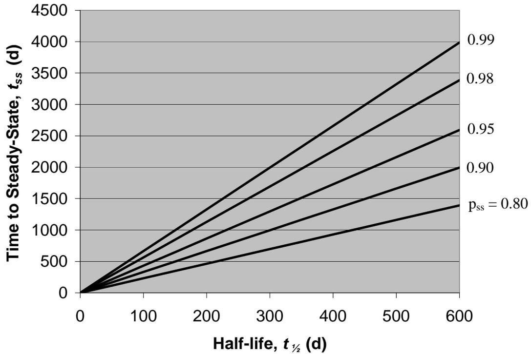
**Fig 2.** Time required to reach approximately steady-state conditions according to Eq. Because ideal steady-state is never actually reached, nutrient budgets may be developed by considering conditions where 95 percent of steady-state is complete.
