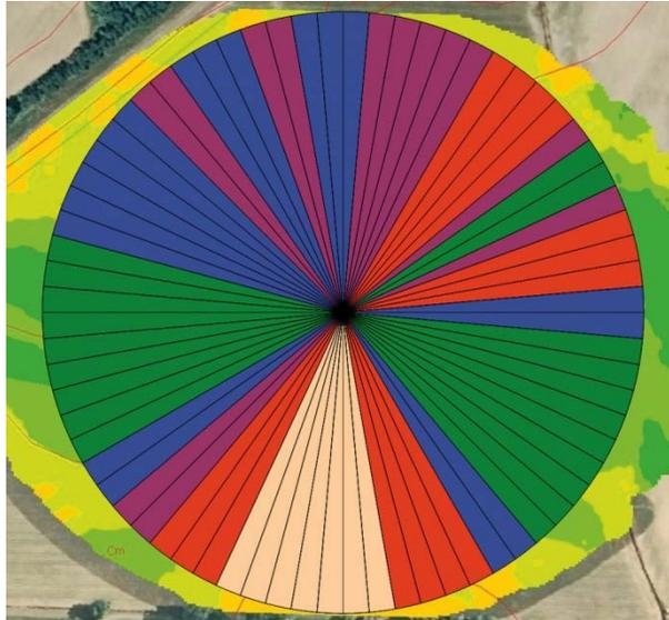
**Figure 1.** Variable Speed Irrigation. The pivot varies travel speed to apply variable amounts of water to defined zones within the field. Colors indicate areas with different amounts of water applied. Image used by permission from [pivotirrigation.com.au](http://pivotirrigation.com.au).
