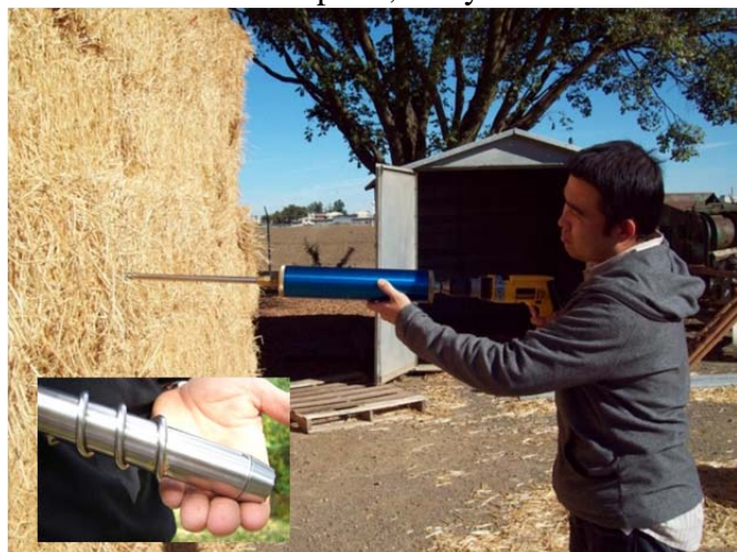
Figure 8. Probes should be taken perpendicular to the butt-ends of bales, so that stems are arranged perpendicular to the probe. Spiral assists and gas-powered drills may assist in penetrating highly-compressed bales.
