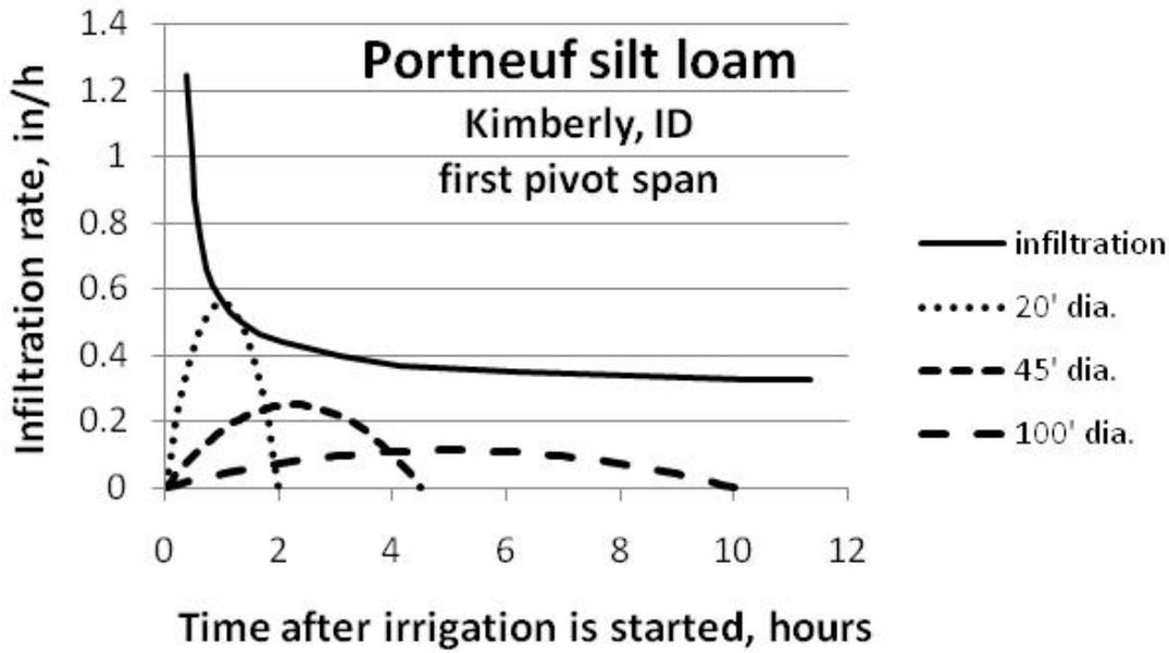
**Figure 3a.** Infiltration rate and water application rate patterns **under the first (inner) span** of a 1300-foot center pivot lateral. Net application rate (assuming 85% application efficiency) is 0.75 for all water application packages. The pivot is operated to make one complete revolution in 2.5 days.
