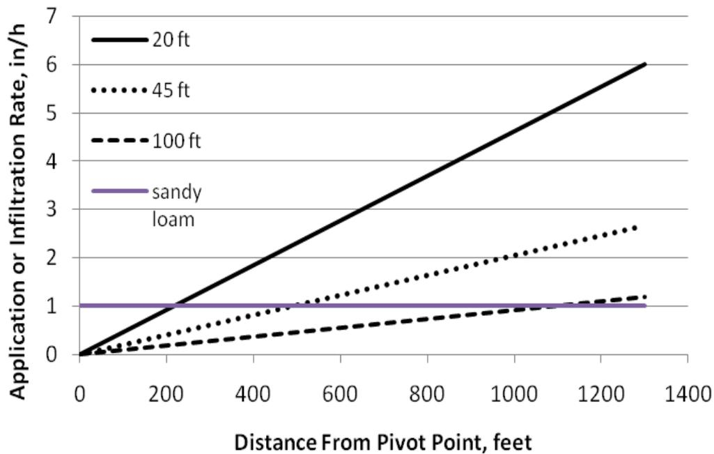
**Figure 4.** Average sandy loam intake rate and average water application rate outward along a center pivot lateral with application package wetted diameters of 20, 45 and 100 feet. Lateral length = 1320 feet and design flow is 850 gpm.
