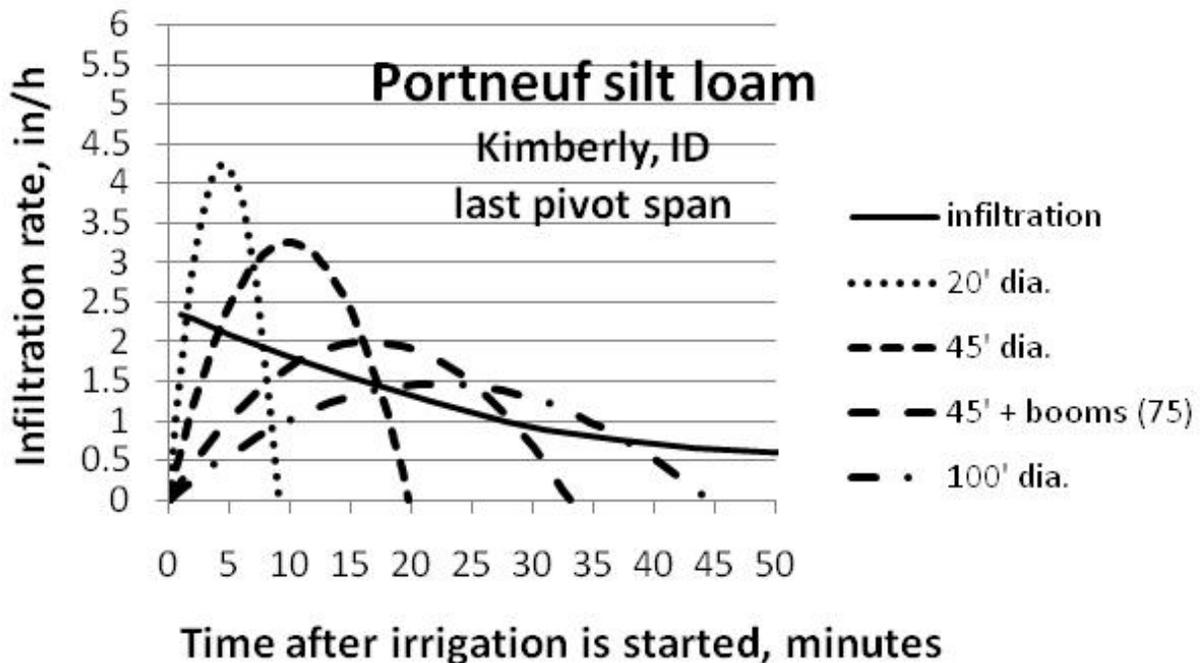
**Figure 3b.** Infiltration rate and water application rate patterns **under the last span** of a 1300-foot center pivot lateral. Net application rate (assuming 85% application efficiency) is 0.75 for all water application packages. The pivot is operated to make one complete revolution in 2.5 days.
