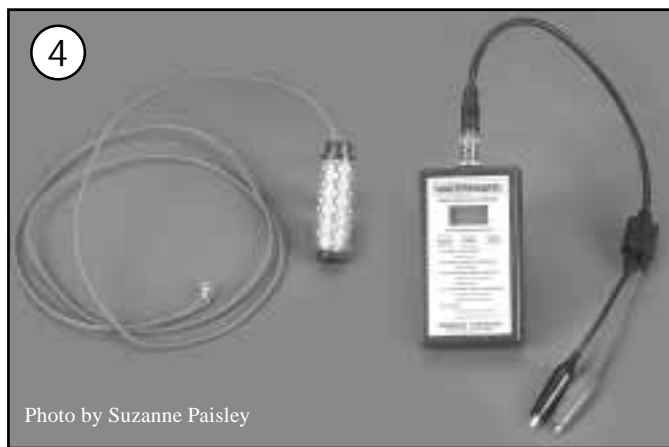
Figure 5. Two sensors at each evaluation site are acceptable but three are preferred because it provides a more complete picture of the soil moisture status at different depths, allowing the irrigator to determine the depth of the last irrigation. For alfalfa install sensors at 1 ft., 2 ft., and 4 ft. (9 inches, 1.5 ft. and 3 ft. in shallow soils). For pasture install sensors at 6 in., 1 ft. and 2 ft.
