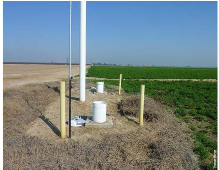
Two monitoring wells (short white casings) adjacent to an irrigated, manure-treated field as part of a dairy monitoring program
