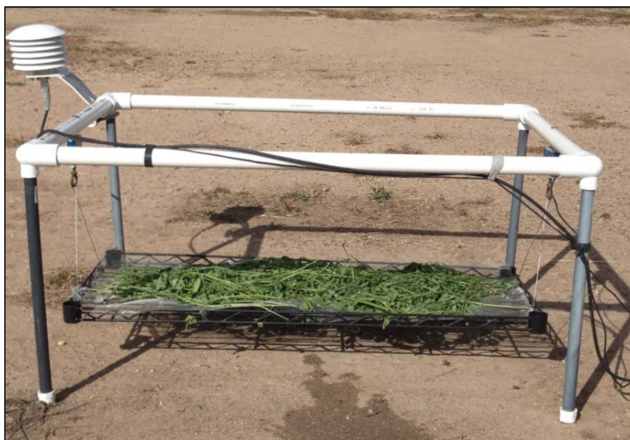
Figure 3. Small, portable field scale used to measure changes in hay moisture after harvest.
