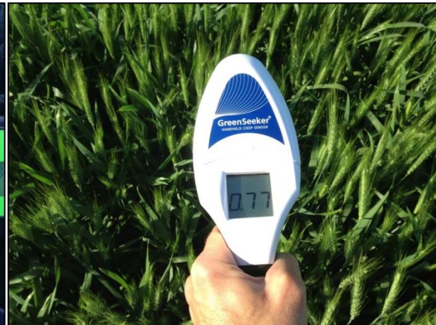
Image B. Greenseeker handheld NDVI meter.
