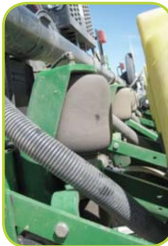
Figure 4. Down pressure airbags on John Deere corn planter.
