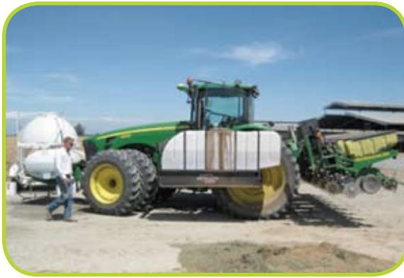
Figure 6. Tractor mounted with liquid fertilizer tanks.
