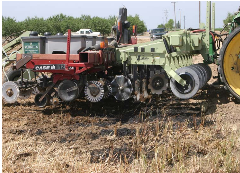
Photo 1 – Orthman 1 tRIPr strip-tiller hooked up with planter for “one-pass” strip- tilling and planting, Kerman, CA, 2006.
