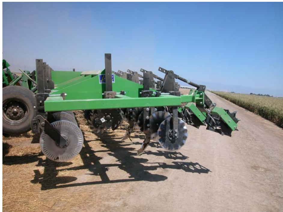
Photo 3. Bigham Brothers Terratill strip-tiller implement close-up showing residue- cutting coulters subsoiling shanks and clod-busting baskets.
