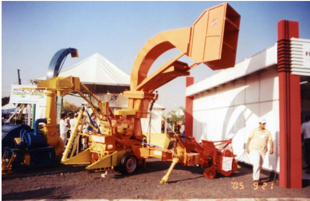
Figure 5: New designed commercial Elephant grass planter and harvester currently being built in Brazil.
