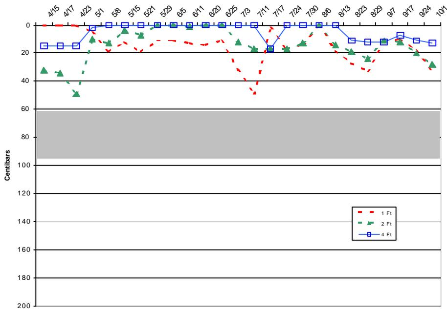
**Figure 3.** Seasonal soil-moisture levels at three depths for over-irrigated alfalfa field. Note that the lines do not fall into the range where irrigation should occur (60–90 centibar zone shaded gray). Irrigations always occurred before Watermark® readings reached this level.
