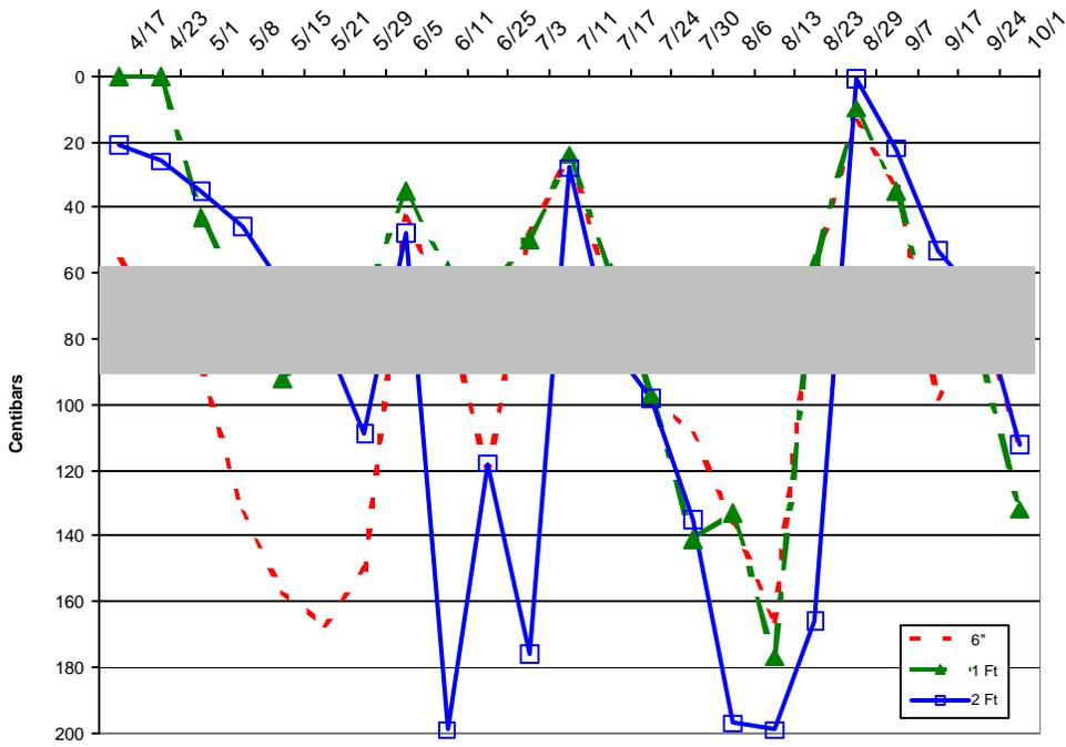
**Figure 2.** Seasonal soil-moisture levels at three depths for sample deficit-irrigated alfalfa field. Note how often the lines fall below the zone where irrigation should occur (60–90 centibar zone shaded gray).
