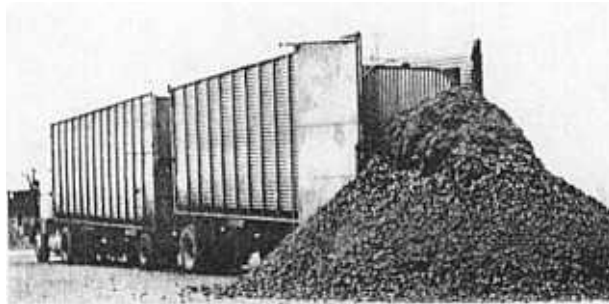
Utilizing fifth-wheel coupler with hydraulic lift so trailer landing gear does not need to be cranked up or down by chopper operator while unloading.
