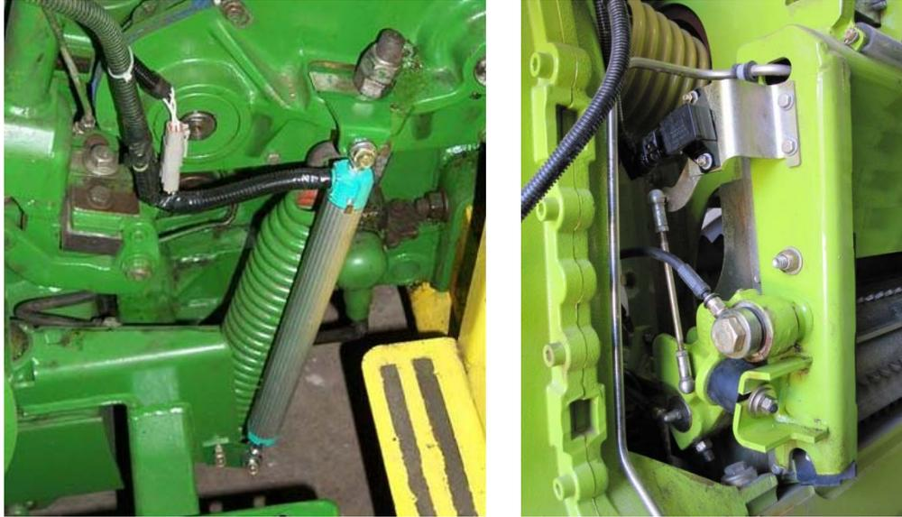
**Figure 2.** Linear (right) and angle (left) sensor for measuring feedroll movement.
