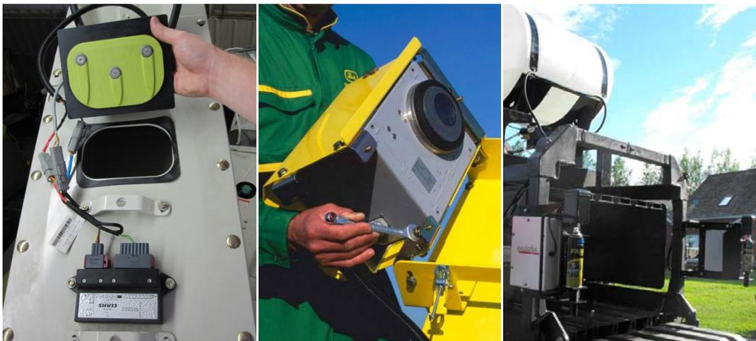
**Figure 3.** Capacitance, near infra-red reflectance and microwave moisture sensors.
